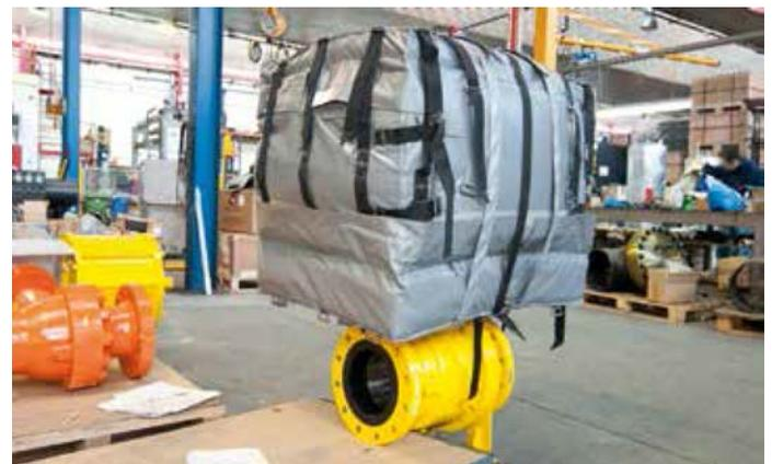
Passive fire protection is a key issue in the safety of hydrocarbon process plants. It is considered a reliable method to reduce plant fire risks. For this matter, BADRAN actuators can be customized to withstand exposure to fire and very high temperatures. A full range of fire proof systems is available, including protective jackets, intumescent coatings and stainless steel enclosure systems.
