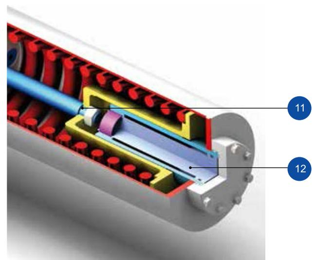
**11** Safe spring Lock, prevents spring module detachment from the drive module
