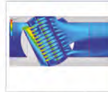
Fig. 2 - CFD showing the velocity reduction inside the trim.
