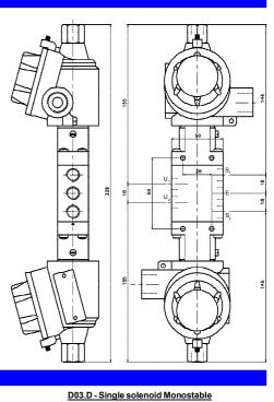
Five way solenoid valve, pilot operated, two and three positions, monostabile or bistable
