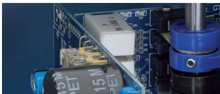
Heating Resistor: •Managed by control board to guarantee the right internal temperature.
